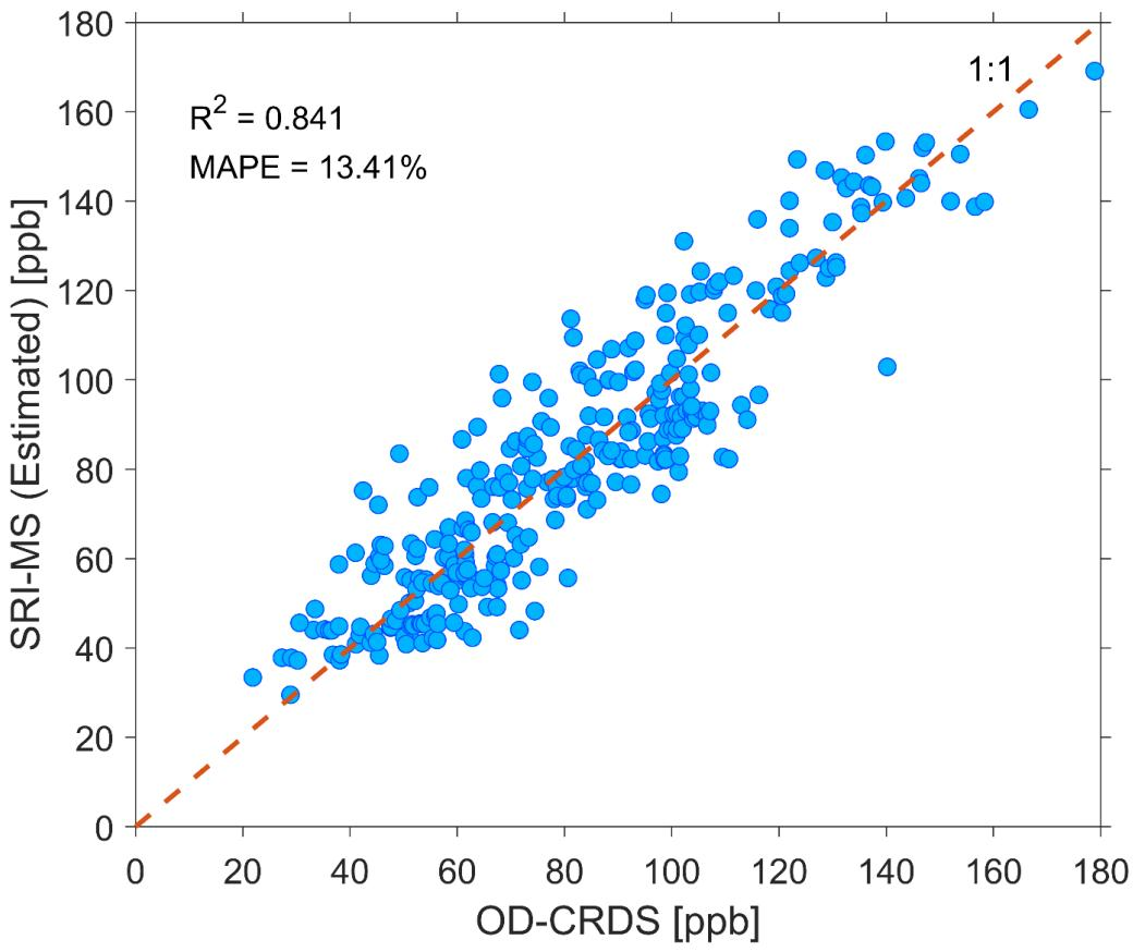
Comparison of the estimated gas-phase  $\text{NCl}_3$  concentration measured by the SRI-MS (assuming a default constant rate coefficient of  $2 \times 10^9 \text{ cm}^3 \text{ s}^{-1}$ ; before applying the correction factors) and the concentration measured by the OD-CRDS (circular marker). The dashed line indicates where the ratio is equal to 1:1. The coefficient of determination ( $R^2$ ) and mean absolute percentage error (MAPE) for the concentrations measured by two instruments are listed.
